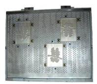
Unique combination of hot-plate/honeycomb fitted in chase. Single-pieced hot plate, 16mm thickness, max area coverage made of high conductivity light alloy. Temperature insulated from machine body for increased energy savings and optimal heat allocation. Moreover, auxiliary materials can be placed underneath the hot-plate in order to achieve simultaneously hotstamping and embossing.
