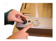
The machine has a compressed air system which allows the regulation of the piston pressure with high accuracy.
