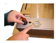
The machine has a compressed air system which allows the regulation of the piston pressure with high accuracy.
