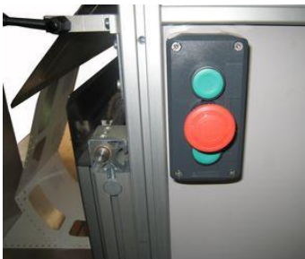
Electrical switch for the control of the delivery pile.
